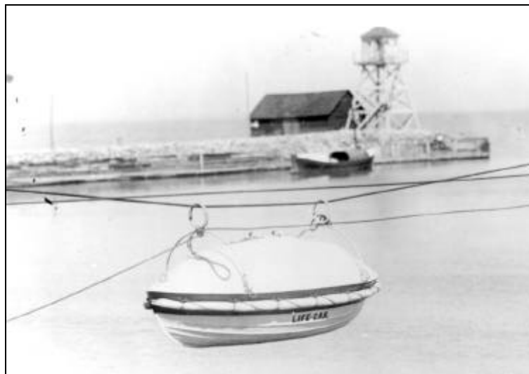
Figure 12. Lifecar Rigged from Ship to Shore. Source: U.S. Coast Guard Headquarters (Life-Saving Service: Surfboats File).
